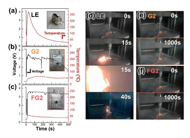
Nail penetration of 650 mAh pouch cells of NCM811llgraphite. (a to c) Voltage and temperature profiles (d to f). Credit: Ulsan National Institute of Science and Technology
