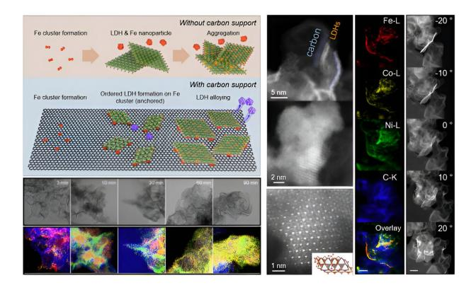
Time-dependent-lapse transmission electron micrograph images of nickel-ironcobalt layered double hydroxide synthesis on carbon support, high resolution scanning TEM and EDS elemental mapping images. Credit: Korea Institute of Science and Technology (KIST)
