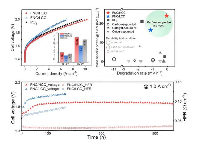
Electrochemical activity evaluation of nickel-iron-cobalt layered double hydroxide and single cell test results. Credit: Korea Institute of Science and Technology (KIST)
