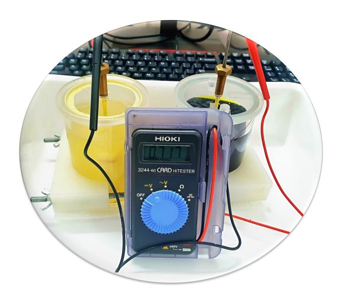
A working MFC using N-S-CNP-based electrodes generating 0.7 V while treating sewage wastewater. Credit: Dr. Shiv Singh
