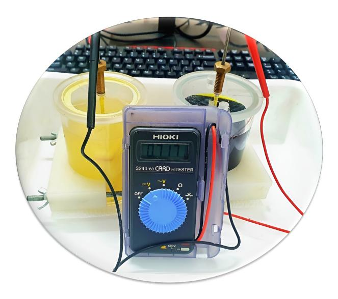
A working MFC using N-S-CNP-based electrodes generating 0.7 V while treating sewage wastewater. Credit: Dr. Shiv Singh
