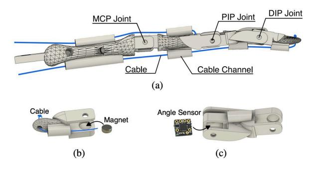
The components of the team's robotic hand. (a) The design of the bones for the index finger is based on the human index finger bones. There are four bones connected with three pin joints. (b) A diametrically magnetized magnet is placed inside the joint of the distal phalange. (c) An angle sensor board is designed and installed inside one joint of the middle phalange. Credit: Liu et al.
