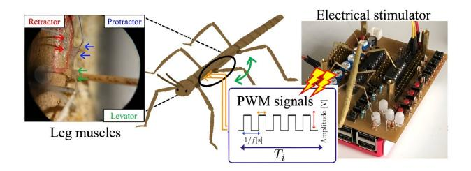
An overview of the experimental setting. Electrical signals were sent to the muscles from the developed electrical stimulation device (right), and the joint torque generated was measured using a force sensor. Electrodes were inserted inside the exoskeleton to transmit electrical stimulation to the three muscles (Protractor, Retractor, and Levator) targeted for electrical stimulation. Credit: Dai Owaki
