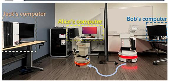
An example of zero-shot interactive personalized navigation. There are three computers in the room never seen by the robot before. The goal is to find Alice's computer. The robot starts by finding the wrong object and needs to communicate with the user and leverage the user feedback to locate the personalized goal. Credit: Dai et al.
