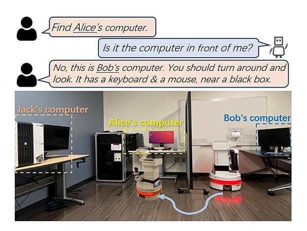
An example of zero-shot interactive personalized navigation. There are three computers in the room never seen by the robot before. The goal is to find Alice's computer. The robot starts by finding the wrong object and needs to communicate with the user and leverage the user feedback to locate the personalized goal. Credit: Dai et al.
