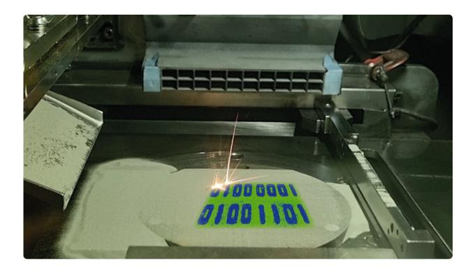
Conceptual illustration showing how the research team's processing strategies can be used to manipulate the structure of metals spatially during laser powder bed fusion processing. Credit: Matteo Seita
