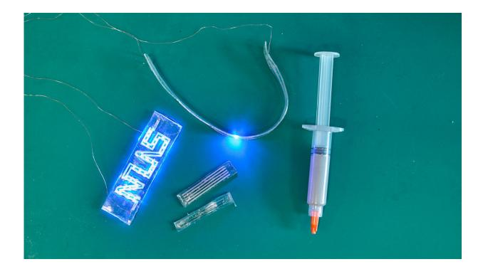
Liquid metal circuitry using a newly engineered material called Bilayer Liquid-Solid Conductor (BiLiSC) allows devices such as wearables to withstand large deformation and even self-heal to ensure electronic and functional integrity. Credit: National University of Singapore
