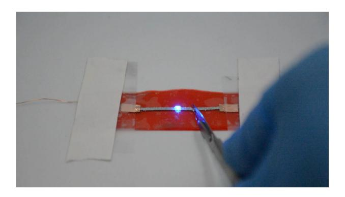
The new conductive and stretchable 'super-material' developed by NUS researchers can heal cracks or cuts almost instantaneously to maintain its electrical conductivity. Credit: National University of Singapore
