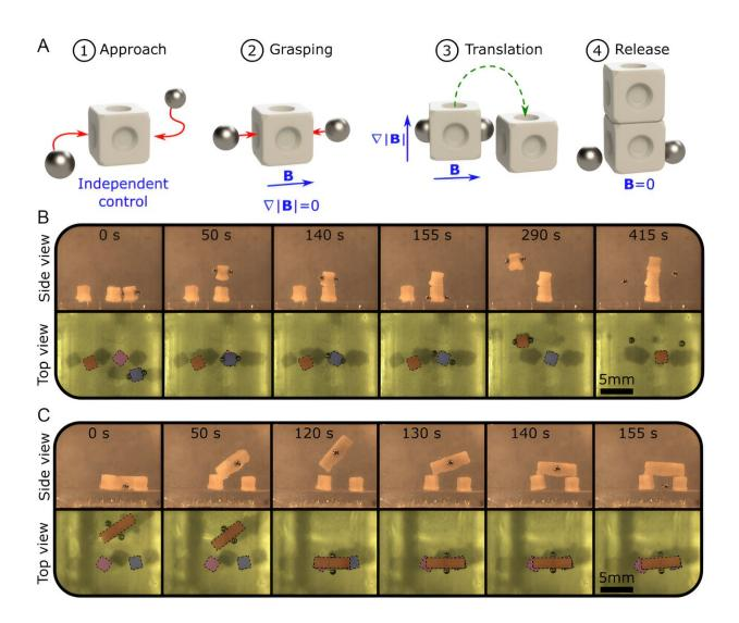
Experimental collaborative grasping and assembly results. The magnetic agents are 1 mm stainless steel spheres and the passive objects are 2 mm 3D printed
