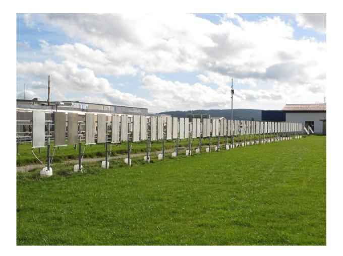
Facade plaster samples were exposed to the elements for 18 months. After each rainfall, they were tested in the laboratory. Credit: Fraunhofer-Gesellschaft
