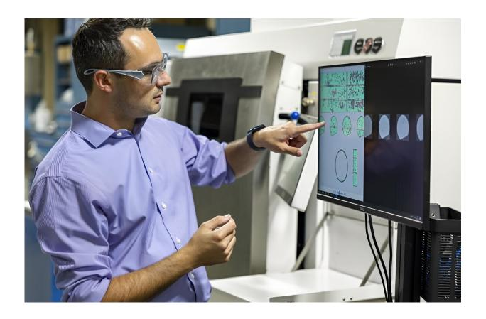
ORNL researcher Zackary Snow compares data from different types of images collected during and after metal parts were additively manufactured using a powder bed printer like the one behind him. Credit: Carlos Jones/ORNL, U.S. Dept. of Energy
