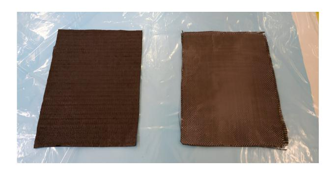
Carbon fibre recycled using the old method (left) compared with Dr He's new method (right). The recycled carbon fibre on the right is stronger and has the potential to be turned into more advanced products. Credit: UNSW Canberra
