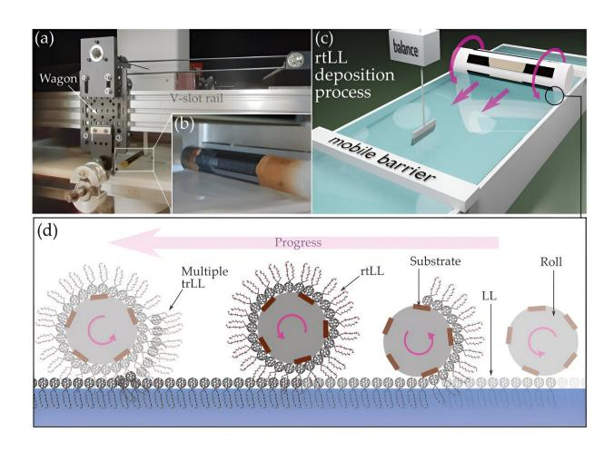
a) Rolling transferred Langmuir layer (rtLL) deposition setup. b) Magnified view of the role with mounted substrates. c,d) Schematic representation of the rtLL deposition process. Credit: *Advanced Materials* (2023). DOI: 10.1002/adma.202305006
