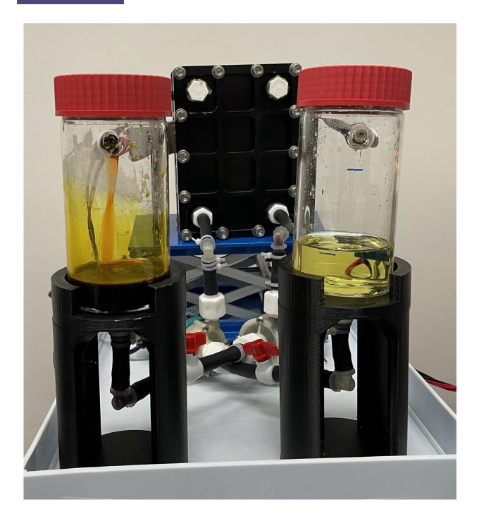
A polysulfide–ferrocyanide redox flow battery stack ( $100 \text{ cm}^2$  with two cells in series) catalyzed by riboflavin sodium phosphate operated at  $100 \text{ mA cm}^{-2}$  (total 10A). Credit: Jiafeng Lei.
