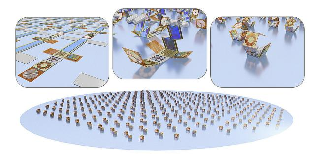
A self-folding microelectronic module (SMARTLET) on a surface that can integrate a wealth of functions, e.g., power supply, actuators, sensors and communication capabilities. Credit: Research Center MAIN, Chemnitz University of Technology
