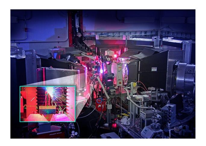
The OpeN-AM experimental platform, installed at the VULCAN instrument at ORNL's Spallation Neutron Source, features a robotic arm that prints layers of molten metal to create complex shapes. This allows scientists to study 3D printed welds microscopically. Credit: Jill Hemman, ORNL/U.S. Dept. Of Energy
