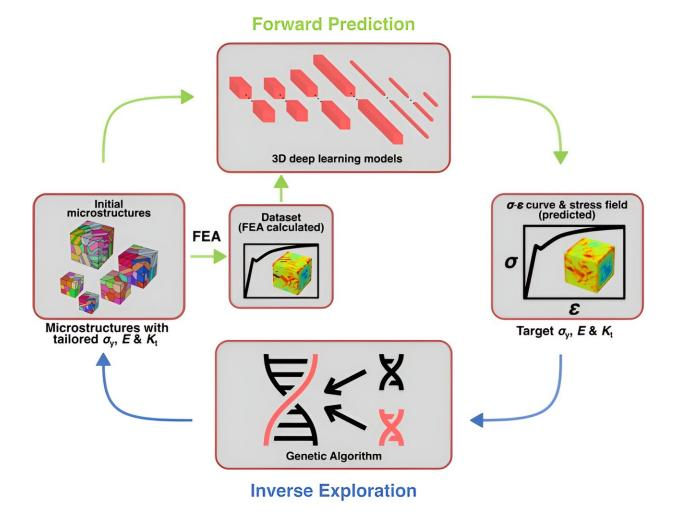
Deep learning models are first established to predict a material's mechanical properties before a genetic algorithm is used to efficiently search for the optimal material microstructure for given target material properties. Credit: Laboratory for Extreme Mechanics and Additive Manufacturing
