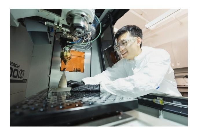
PhD candidate Xiao Shang operates the directed energy deposition 3D printer that was designed and built in the metal additive manufacturing lab of Assistant Professor Yu Zou. Credit: Neil Ta
