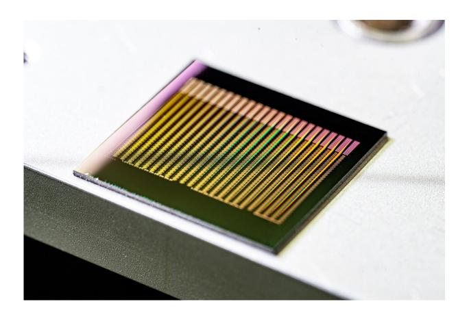
The chip contains almost 8,400 functioning artificial neurons from waveguide-coupled phase-change material. Credit: Jonas Schütte / AG Pernice
