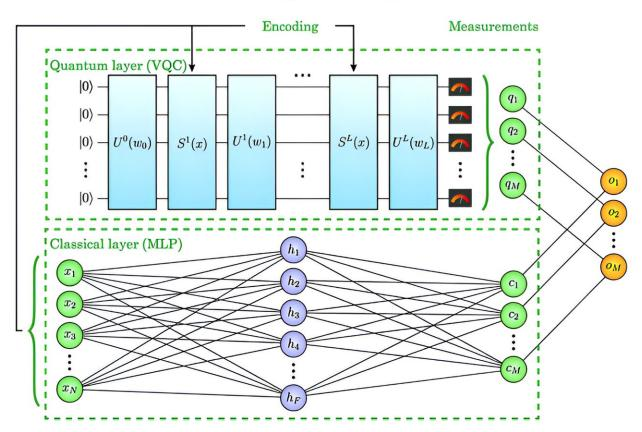
The model takes the input and simultaneously feeds it into the quantum layer and the classical layer for parallel processing before combining the outputs of both layers to produce the final output. Credit: MO KORDZANGANEH ET AL.
