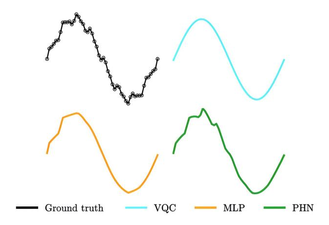
The quantum layer (a variational quantum circuit or VQC) and the classical layer (a multi-layered perceptron or MLP) each do a worse job of modeling the data than the two layers do when they are combined in a parallel hybrid network (PHN). Credit: MO KORDZANGANEH ET AL.
