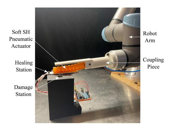
The automatic robotic system for testing the healability of pneumatic SH actuators. Characterization of the actuator continuously occurs as it is repeatedly damaged at the "Damage Station" and repaired at the "Healing Station." SH, self-healing. Credit: *Robotics Reports* (2023). DOI: 10.1089/rorep.2023.0014
