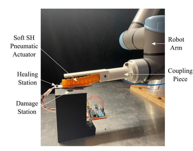
The automatic robotic system for testing the healability of pneumatic SH actuators. Characterization of the actuator continuously occurs as it is repeatedly damaged at the "Damage Station" and repaired at the "Healing Station." SH, self-healing. Credit: *Robotics Reports* (2023). DOI: 10.1089/rorep.2023.0014
