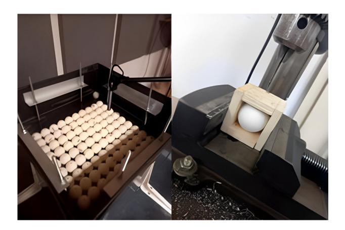
Experimental setup and numerical model of sound transmission through an acoustic metasurface based on pierced pingpong balls. Credit: Sabat et al.
