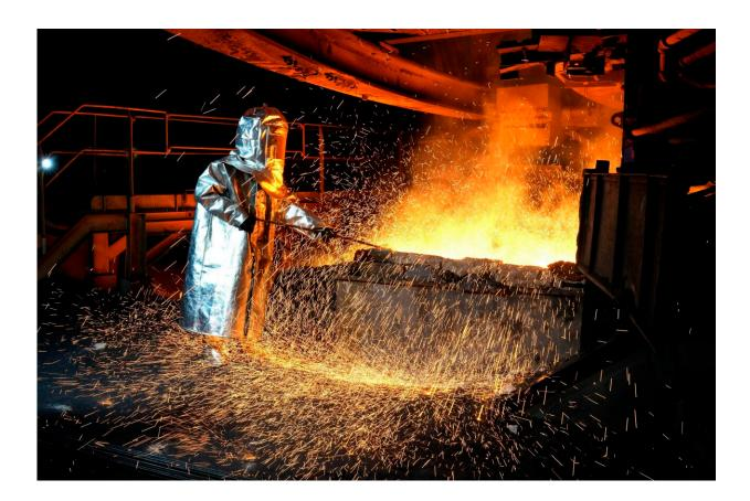
A worker in a protective suit pokes a metal rod to tap slag from a smelting furnace at PT Vale Indonesia's nickel processing plant in Sorowako, South Sulawesi, Indonesia, Tuesday, Sept. 12, 2023. As demand for materials needed for batteries, solar panels and other components vital for cutting global emissions rises, carbon emissions by miners and refiners will likewise rise unless companies actively work to decarbonize. Credit: AP Photo/Dita Alangkara
