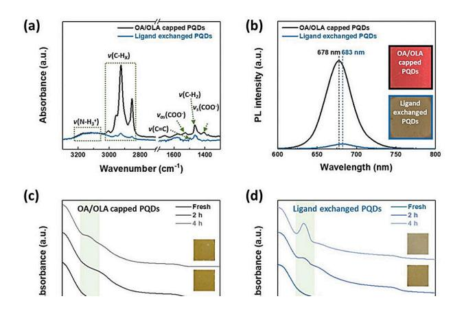
a) FT-IR and b) PL spectra of the OA/OLA-capped and ligand-exchanged PQD solids, respectively. The insets in b exhibit photographs of each PQD solid under UV irradiation. UV–vis absorbance spectra and photographs of c) OA/OLA-capped and d) ligand-exchanged PQD solids before and after storing under harsh relative humidity of 50–60% RH condition. e) Schematic illustration of conventional ligand exchange procedure. Credit: *Advanced Science* (2023). DOI:
