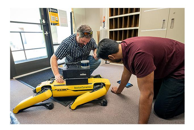
Brian Quiter (left) and Kushant Patel test the physical coupling of a radiation imaging system with a Boston Dynamics Spot Robot. Credit: Thor Swift/Berkeley Lab
