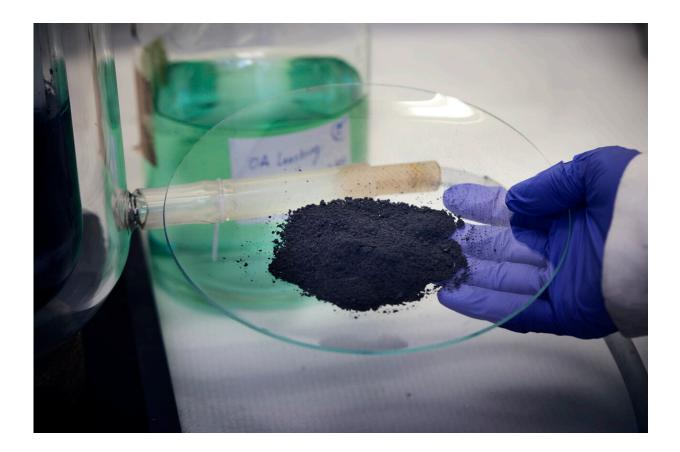
After the aqueous-based recycling method, the aluminum and lithium end up in the (greenish blue) liquid. The other metals, such as cobalt, nickel and manganese, remain in the dark "solids", shown on the plate. Credit: Chalmers University of Technology | Anna-Lena Lundqvist
