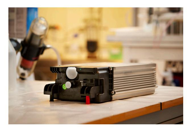
The researchers at Chalmers work with real spent car batteries from Volvo Cars. Here is a battery module, holding 14 battery cells. Credit: Chalmers University of Technology | Anna-Lena Lundqvist
