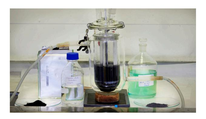
How the method works: the crushed contents of a spent car battery cell (silver bag), in the form of a finely ground black powder (dish on the left), are dissolved in a transparent liquid – oxalic acid. After a set time, the black mixture is filtered. The aluminum and lithium end up in the (greenish blue) liquid, while the other metals, such as cobalt, nickel and manganese, remain in the dark "solids" (dish on the right). Credit: Chalmers University of Technology | Anna-Lena Lundqvist
