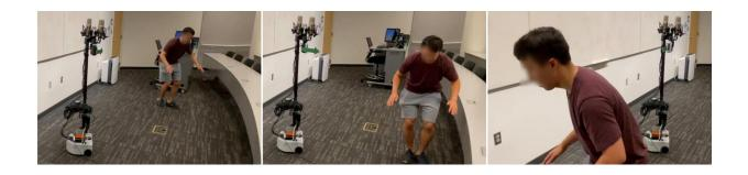
The robot tracks the person using only the subtle incidental sounds created as they move quietly. The robot rotates the attached green arrow to face where the model estimates the person to be. Credit: Georgia Institute of Technology.
