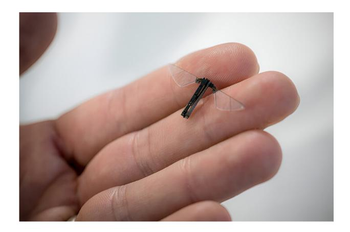
Expirements on this tiny robot helped researchers better understand how asynchronous flight has evolved. Credit: Erik Jepsen/University of California San Diego
