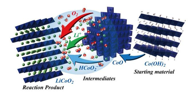
Reaction pathway of the hydroflux process to form layered lithium cobalt oxide (LiCoO<sub>2</sub>) at 300 °C. Credit: *Inorganic Chemistry* (2023). DOI: 10.1021/acs.inorgchem.3c01704
