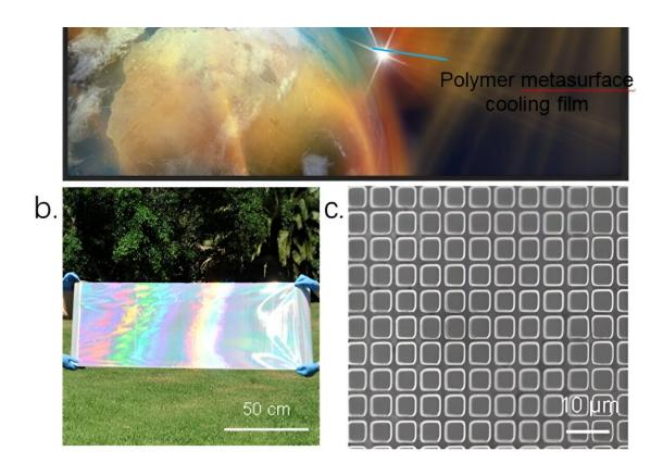
Concept and demonstration of polymer metasurface radiative cooling film. a. Conceptual image of the large-scale polymer metasurface cooling down the Earth under sunlight. b. A photo of the large-scale and flexible polymer metasurface cooling film. c. An SEM image of the microstructures in the polymer metasurface cooling film. Credit: TranSpread
