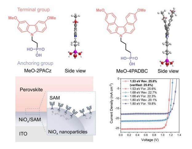
Molecular structure of the novel SAM, schematic illustration of SAM deposition method, and photovoltaic performance of SAM-based perovskite solar cells. Credit: Professor Zhu Zonglong's research group / City University of Hong Kong
