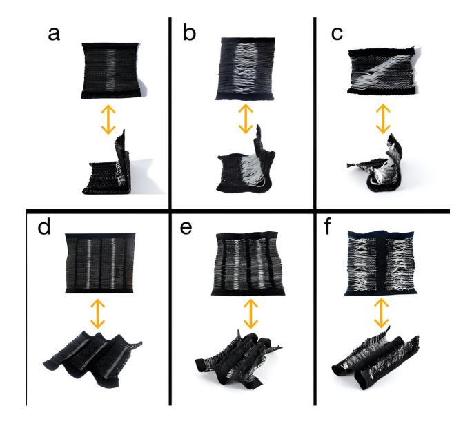
The fiber contracts in response to an increase in temperature, then self-reverses when the temperature decreases, without any embedded sensors or other hard components. Credit: Massachusetts Institute of Technology
