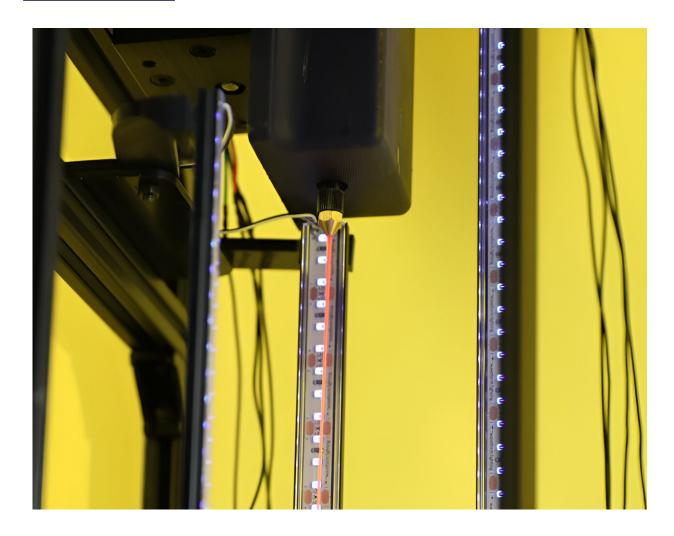
Researchers used a material known as liquid crystal elastomer (LCE). The thick and viscous LCE resin is heated, and then slowly squeezed through a nozzle like that of a glue gun. As the resin comes out, it is cured carefully using UV lights that shine on both sides of the slowly extruding fiber. Credit: Massachusetts Institute of Technology
