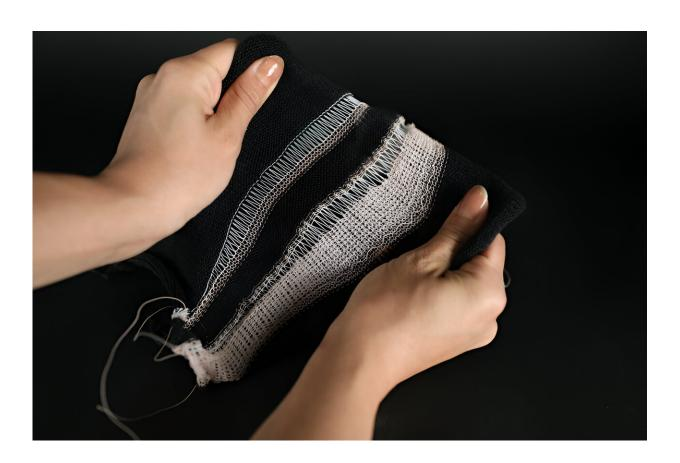
Researchers from MIT and Northeastern University developed a liquid crystal elastomer fiber that can change its shape in response to thermal stimuli. The fiber, which is fully compatible with existing textile manufacturing machinery, could be used to make morphing textiles, like a jacket that becomes more insulating to keep the wearer warm when temperatures drop. Credit: Massachusetts Institute of Technology
