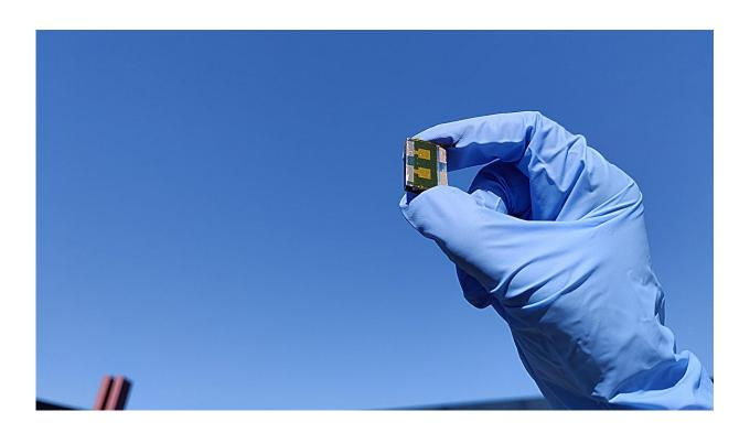
An inverted perovskite solar cell with a new design of hole-selective contacts. Credit: EPFL Felix T. Eickemeyer—CC-BY-SA 4.0
