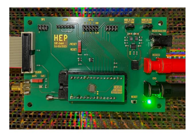
The security chip (at the middle of the bottom) is built in flip-chip technology on an auxiliary board and plugged into a standard socket on the main board. The main board handles communication with other components. Credit: Franziska Wegner
