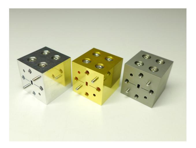
Researchers fabricated 20mm length waveguides made of the superconducting metal niobium (right). It shows improved conductivity compared with normal metal materials such as a gold-plated tellurium copper (middle) and aluminum alloy (left), and can transmit radio waves that are necessary for B5G/6G
