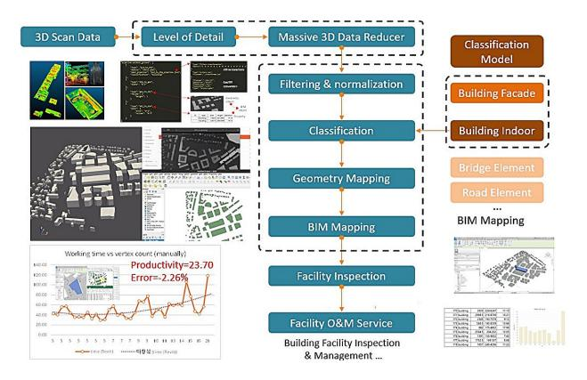
The Scan to BIM pipeline we are working on normalizes the reverse engineerin engineering process into task units so they can? be assembled. Reverse engineering tasks are predefined, including LoD processing, classification, and geometry generation. This technology provides Scan to BIM Description Language (SBDL) to connect and assemble tasks. Credit: Korea Institute of Civil Engineering and Building Technology(KICT)
