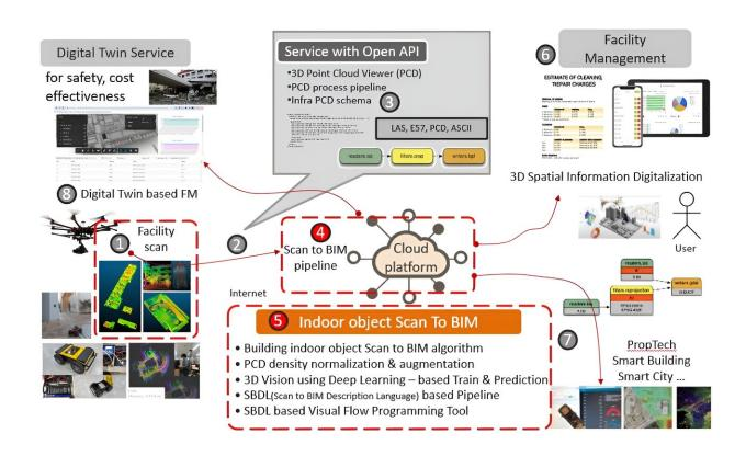
Scan data collected from rovers, drones, lidar, etc. is automatically processed through the Scan to BIM pipeline to generate the information desired by the user. This spatial information digitization technology can be used in digital twin-related services that use spatial information. Credit: Korea Institute of Civil Engineering and Building Technology(KICT)
