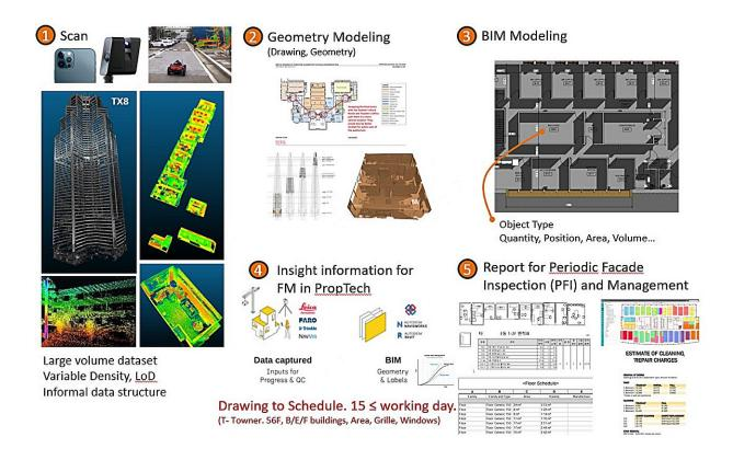
This R&D project believes that indoor and outdoor scan data can be used for facility maintenance and operation, construction management, infrastructure quality inspection, and proptech asset digitization. Using Scan to BIM automation technology, we can extract the desired quantities from scan data, which is a simple point data, and obtain the dimensions of the object quickly. Credit: Korea Institute of Civil Engineering and Building Technology(KICT)
