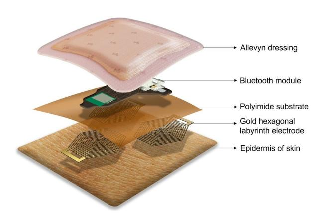
An artist's impression of the RMIT ECG device, showing the various layers including a dressing, Bluetooth module and dry electrodes. Credit: RMIT University
