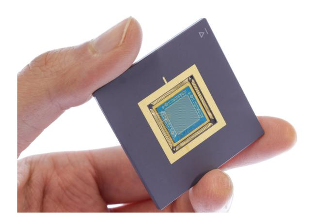
In a paper published in the journal *Nature Electronics*, researchers from EPFL's School of Engineering in the Laboratory of Nanoscale Electronics and Structures (LANES) present a new processor that tackles this inefficiency by integrating data processing and storage onto a single device, a so-called in-memory processor. They broke new ground by creating the first in-memory processor based on a two-dimensional semiconductor material to comprise more than
