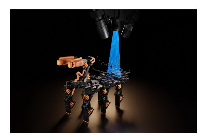
A new high-throughput, multimaterial 3D inkjet printer uses computer vision to rapidly and automatically control the amount of material being printed in real-time. This rendering shows a robot being built layer-by-layer using the process. The black spheres represent the material that the printer uses. The material is then cured by UV light, represented in blue. At the top of the image are the cameras that scan the procedure and adjust accordingly. Credit: Moritz Hocher
