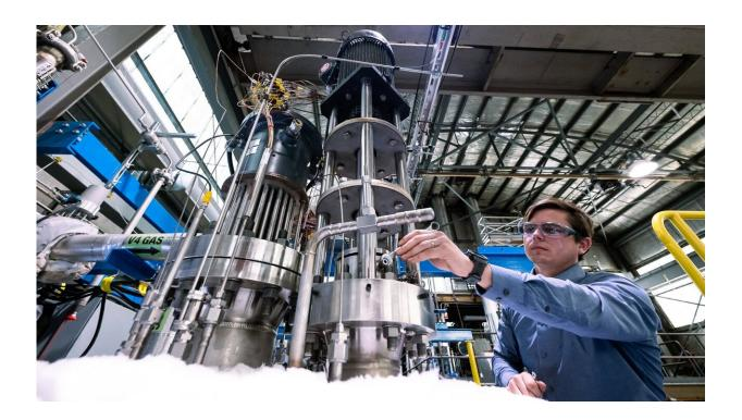
Argonne's machine learning model is equipped to analyze data from 31 sensors at its Mechanisms Engineering Test Loop (METL) facility, measuring variables like fluid temperatures, pressures and flow rates. Credit: Argonne National Laboratory
