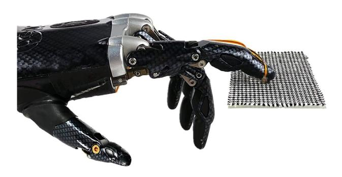
Texture recognition by slipping the slip sensor on a textile. Credit: Chuan Fei Guo
