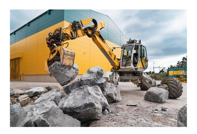
The Menzi Muck picks and scans each boulder to be placed in the correct position, Circularity Park in Oberglatt, Eberhard AG, 2021–2022. Credit: Gramazio Kohler Research, ETH Zurich, Eberhard AG. Photo: Marc Schneider.
