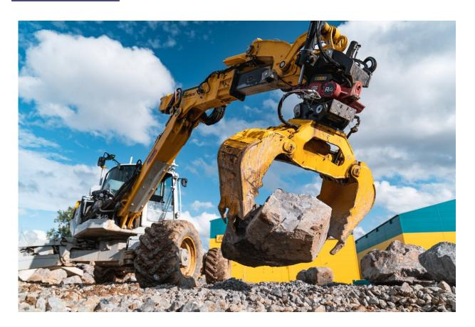
The Menzi Muck picks and scans each boulder to be placed in the correct position, Circularity Park in Oberglatt, Eberhard AG, 2021–2022. Credit: Gramazio Kohler Research, ETH Zurich, Eberhard AG. Photo: Marc Schneider.
