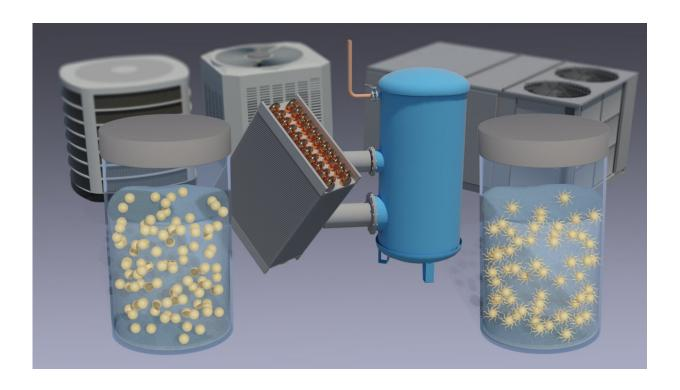
ORNL researchers found that a polyelectrolyte additive can improve the stability and performance of a salt hydrate PCM, enhancing the potential for use in heat pumps. Credit: ORNL, U.S. Dept. of Energy
