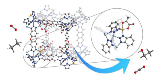
Detail of the porous MOF (left and inside circle at right) showing the metal reactive site where oxygen and hydrocarbons like ethane (molecules at extreme left) are converted into alcohols, such as ethanol, plus carbon dioxide (molecules at extreme right). The red balls are oxygen atoms; the gray are carbon; yellow is iron; light blue is zinc; dark blue is nitrogen; and white is hydrogen. Credit: Jonas Börgel/UC Berkeley
