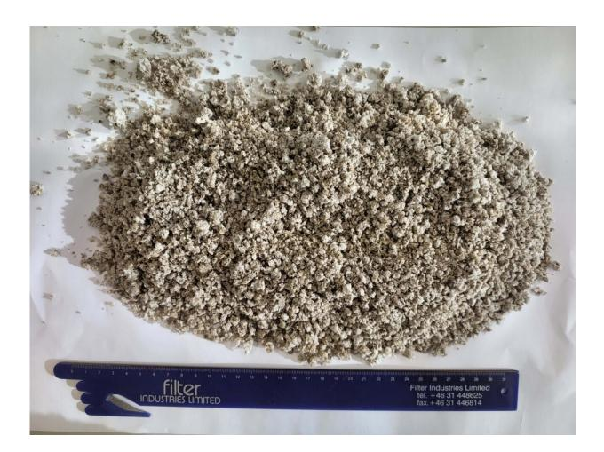
This is the powdered SiGS slag that can act as a substitute for cement in concrete. Credit: SINTEF
