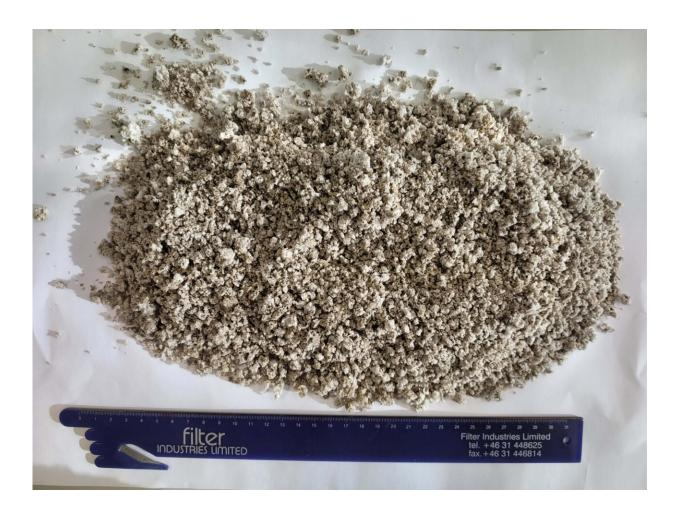
This is the powdered SiGS slag that can act as a substitute for cement in concrete. Credit: SINTEF
