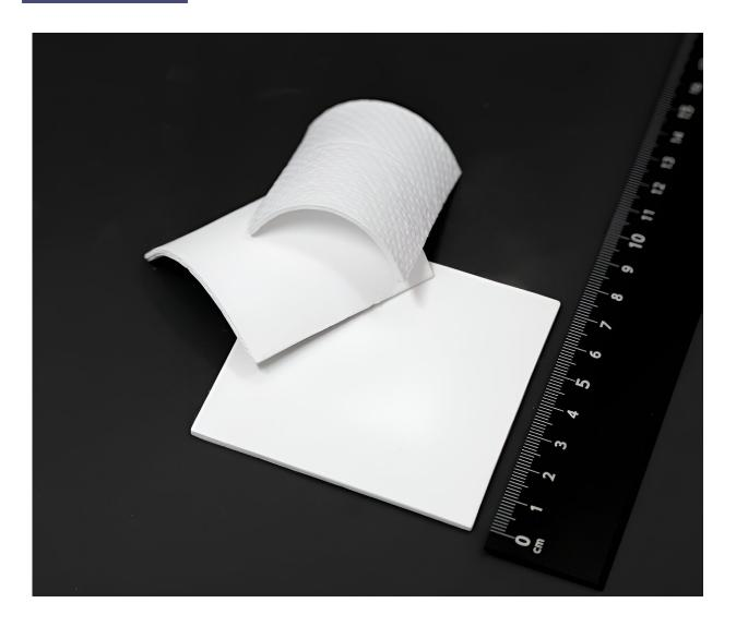
Cooling ceramics with flat and curved shapes. Patterns can be applied on the cooling ceramic surface. Credit: City University of Hong Kong
