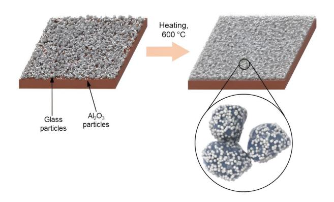
Schematic of the fabrication of the radiative cooling glass coating. By heating to ~600°C, the low-melting-point glass microparticles in the mixture can be rapidly sintered to form an interconnected mesoporous structure. Credit: *Science* (2023). DOI: 10.1126/science.adi2224
