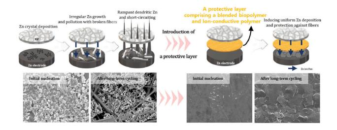
Introducing a xanthan gum-based shield to drive uniform zinc deposition. Credit: POSTECH
