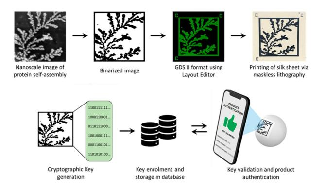
Schematic showing the proposed process for image PUF generation and printing. Credit: *Micromachines* (2023). DOI: 10.3390/mi14091678
