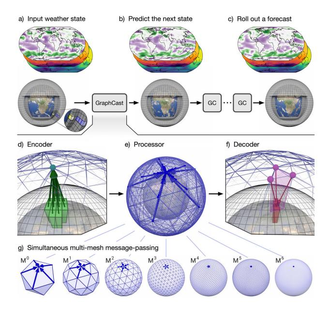
Model schematic.(A) The input weather state(s) are defined on a 0.25° latitude-
