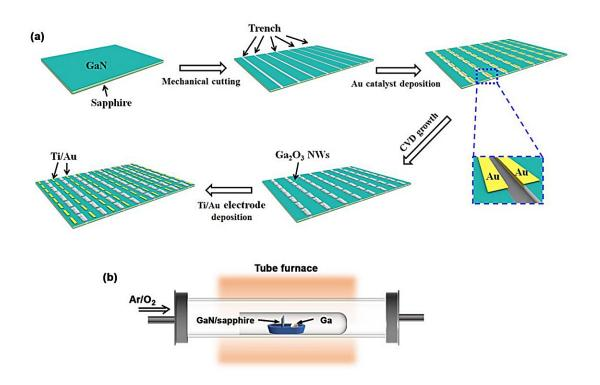
a) Stepwise procedure for the fabrication of the GaN/Ga<sub>2</sub>O<sub>3</sub>/GaN TB heterostructure array device. b) Schematic diagram of the experimental set-up for the CVD synthesis of Ga<sub>2</sub>O<sub>3</sub> TB NWs. Credit: *Advanced Materials* (2023). DOI: 10.1002/adma.202308090
